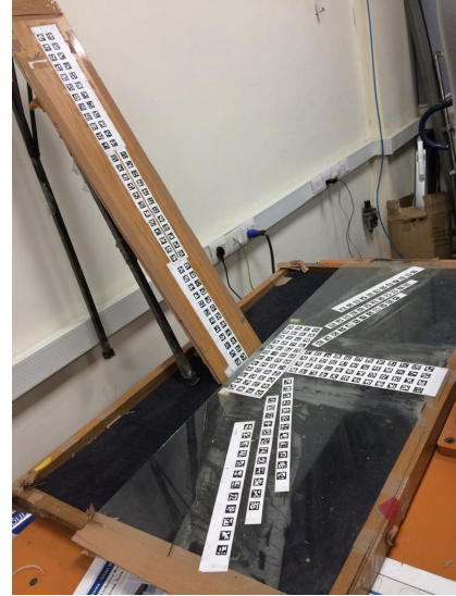
Figure 3: ArUco markermap bed consisting of 216 6x6 bit ArUco markers
