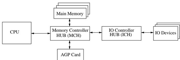
Figure 1: Intel chipset architecture.
