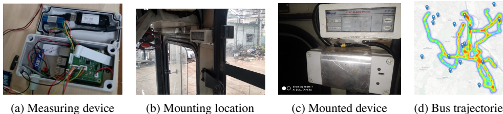
Figure 1: (a) Inside of our PM measuring IoT unit. (b) Mounting location in bus driver's cabin in non air-conditioned public bus (below the existing white box). (c) Mounted IoT unit in the bus (below the existing white box). (d) Government deployed static sensors installed in and around our bus trajectories, as location icons.
