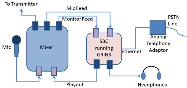
Fig. 2. A radio station setup using GRINS: The single board computer (SBC) running GRINS is connected to the mixer, which is in turn connected to the transmitter. Telephony adaptor allows connecting PSTN line to the SBC
