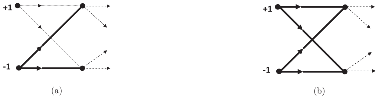
Figure 6.4: (a) MLSD for P-DS, and (b) Modified MLSD for P-DSA (The bold lines represent the possible paths emanating from the initialization state).
