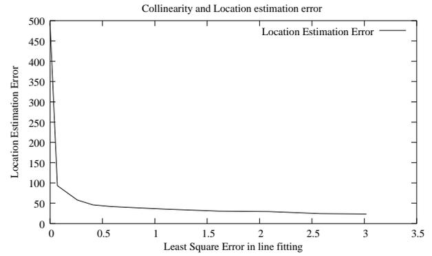
Fig. 5. Effect of collinearity on location estimation error
