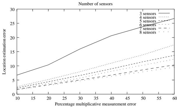
Fig. 1. Measurement error vs. Location estimation error
