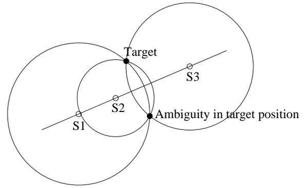
Fig. 4. Ambiguity in target location in case of collinear sensors
