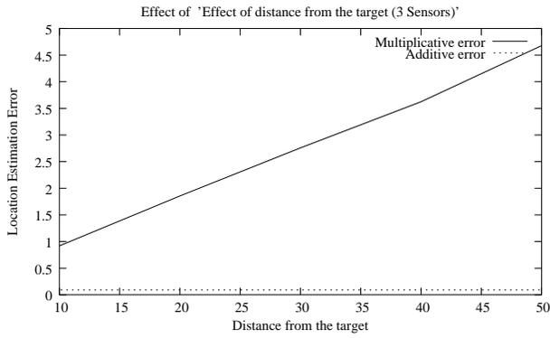
Fig. 10. Effect of distance on location estimation error
