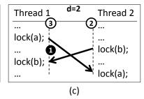
Figure 6: Illustration on how our randomized scheduler finds bugs of depth d, using the examples from Fig. 1. The scheduler assigns random initial thread priorities  $\{d,\ldots,d+n-1\}$  (white circles) and randomly places d-1 priority change points of values  $\{1,\ldots,d-1\}$  (black circles) into the execution. The bug is found if the scheduler happens to make the random choices shown above.
