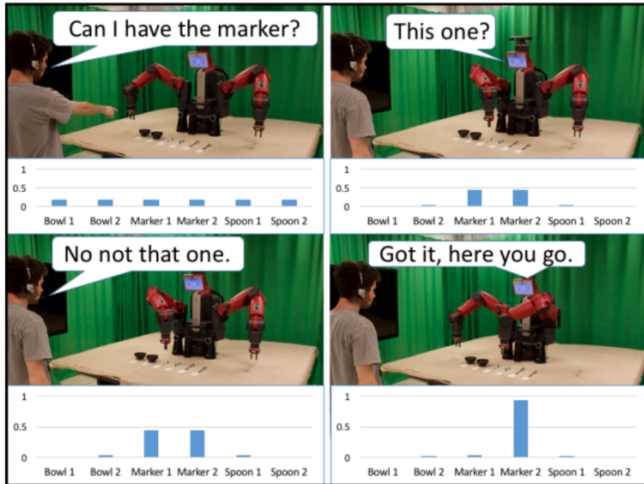
Fig. 1. Demonstration of our FETCH-POMDP model correctly fetching item for user. Note the robot's understanding of implicit information between panels three and four. This reasoning is not hard-coded into our system, but emerges from the solution of our POMDP.
