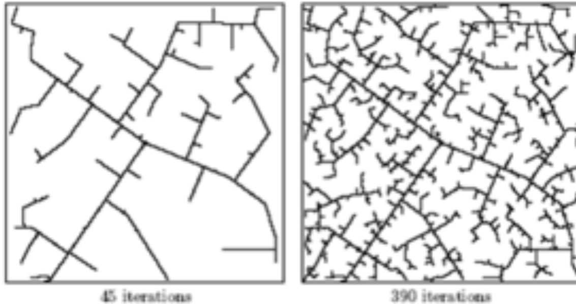
A visualization of an RRT graph after 45 and 390 iterations
