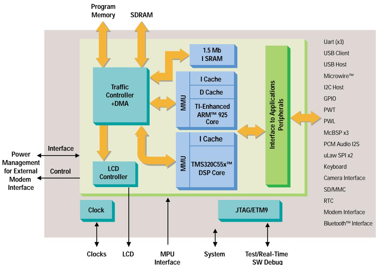
ing a large memory space for power efficient on-chip data and code storage for applications such as liquid crystal display (LCD) frame buffering. A two level interrupt handler provides 32 interrupt lines including 13 internal and 19 external interrupts. Also included in the core is the ARM CP15 coprocessor and protection module.
