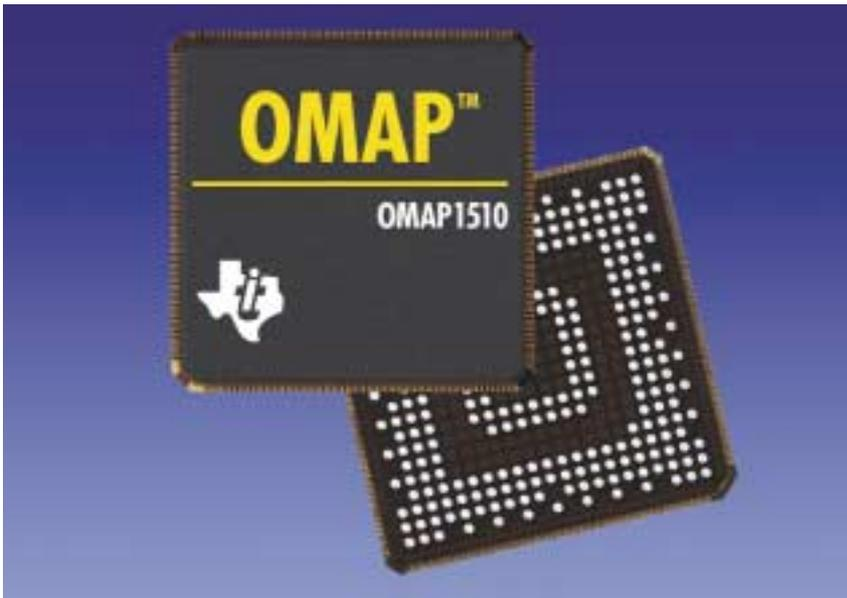
*The OMAP1510 processor is a unique dual-core architecture that combines the command and control capabilities of the TI-enhanced ARM™ 925 processor with the high-performance and low power capabilities of the TMS320C55x™ DSP core.*
