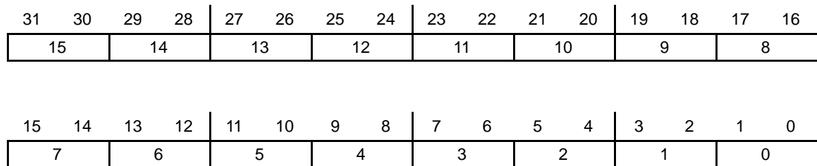
Figure 2–19. Domain Access Control Register Format
