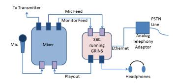
Fig. 2. A radio station setup using GRINS: The single board computer (SBC) running GRINS is connected to the mixer, which is in turn connected to the transmitter. Telephony adapter allows connecting PSTN line to the SBC
