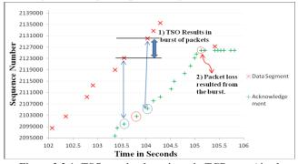
Figure 2.2.1: TSO causing burstiness in TCP over Airtel HSDPA connection in downlink direction.
