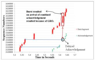
Figure 2.2.2: Combined acknowledgement causing burst in flow over Airtel HSDPA connection in downlink direction.
