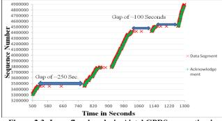
Figure 2.3: Long flow breaks in Airtel GPRS connection in downlink direction.
