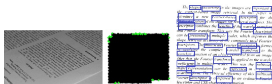
Fig. 9. Figure showing the performance of the proposed technique on a highly skewed query image. From left-to-right, the original query image; its binarised version; and the contour with its prominent curvature extrema points
