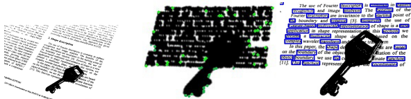
Fig. 11. Successful matching in spite of structured noise/occlusion, and some skew as well. Unlike Fig. 10 where the zig-zag (word bounding box) feature is affected by occlusion, in this case, both the contour extrema feature and the zig-zag feature are affected. Our probabilistic information fusion strategy enables successful recognition, again.
