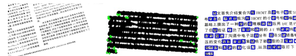
Fig. 14. A case of failure, when the near-failure of a particular feature pulls down the overall probability. For the sake of illustration, we tweaked the bounding box size threshold. For this Chinese language document, the word bounding box feature does not work properly, owing to insufficient word-character separation. (Sec. 5.3)
