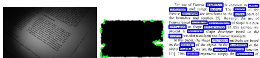
Fig. 6. The system works in cases of bad illumination (here, there is considerable skew as well): an example. The figure shows (left-to-right), the input image; the contour extrema features on the prominent text block; and the zig-zag (word bounding box) features. In both cases (as with all other results), the query block is relatively ‘straightened’ as the features map the given possibly skewed query image block, to a database document image block, which is in a canonical skew-less orientation. Details in Sec. 5.1.
