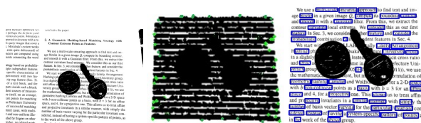
Fig. 10. Successful matching in spite of structured noise/occlusion. In this case, the zig-zag word bounding box) feature is affected by the occlusion, but the feature (contour extrema) is relatively unaffected by it. Our probabilistic information fusion strategy enables successful recognition.
