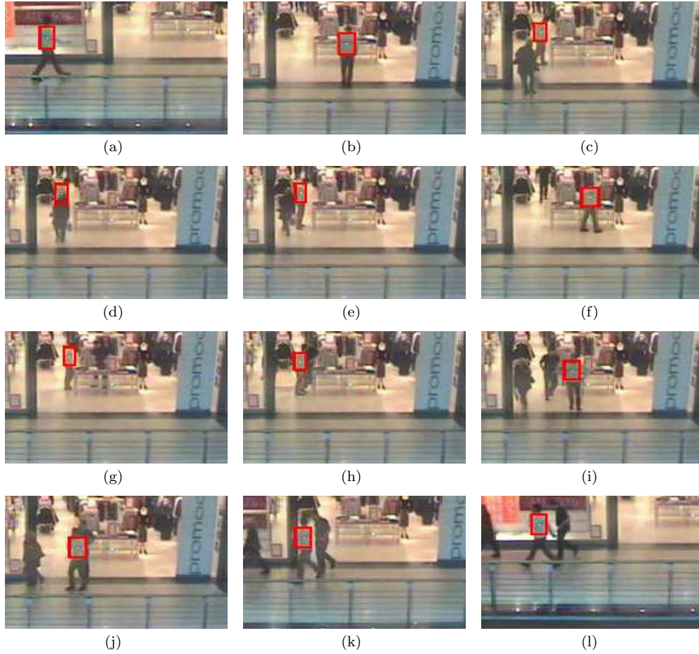
FIG 2. Caviar Sequence: The object to be tracked is very small and has same colour as the background. There are multiple moving objects and occlusion is also handled well.
