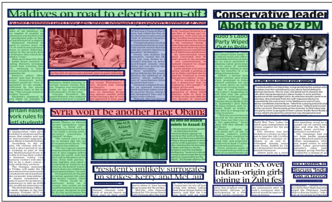
Fig. 2. Neighborhood Selection: Current block marked in blue, neighbors at m = 1 marked in red, neighbors at m = 2 marked in red and green
