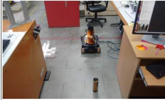
Figure 1: Experimental Setup: Demonstrating a YouBot and an object lying in front of the youBot, that is to be picked.
