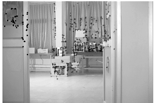
Figure 2: Corner matches between views 1 and 3 corresponding to the three planar patches. The matches corresponding to each patch are shown with different symbols.
