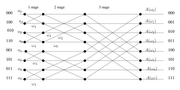
Figure 7.1: Computing an eight point FFT using a butterfly network
