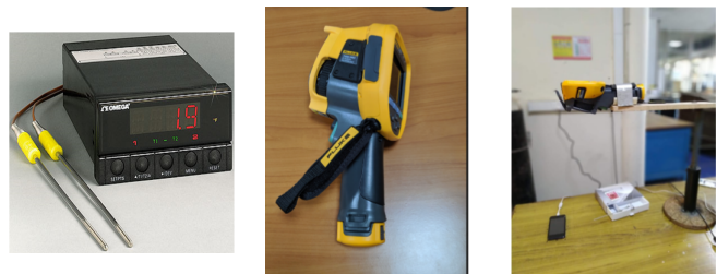
Fig. 2: Devices used and the setup for calibration (a) Digital Temperature Sensor (b) Thermal Imaging Camera (c) Experimental setup
